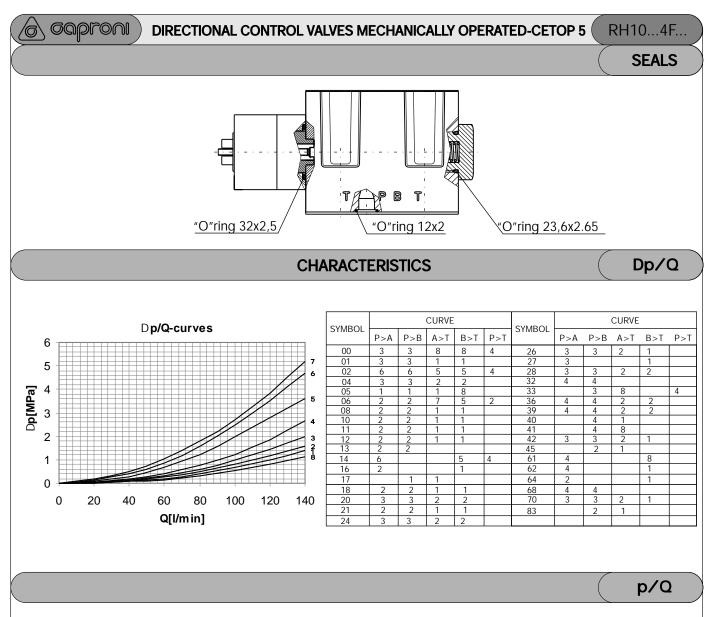
The operating limit of hydraulic power shown here is for applications with two directions of flow (e.g. from P to B and simultaneously from A to T). If the valve is with one direction passage only (e.g. from P to B and with blocked port A), the operating limit may considerably be reduced. The performance limits are measured with hydraulic oil  $35\pm5$  cSt and temperature 50 °C.
